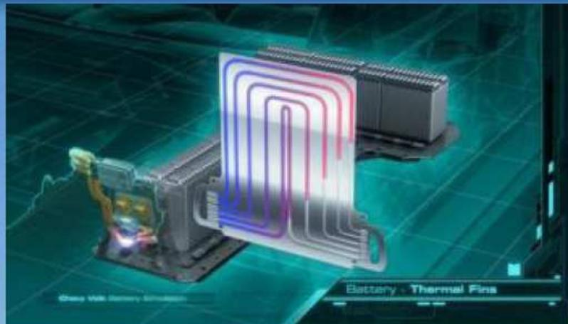
Cooling fin concept enables effective heat exchange to/from Lithium Ion pouch cells
